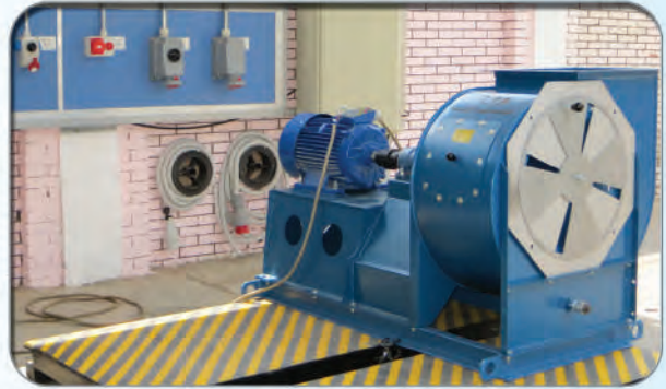
Test Station for all fans before delivery
