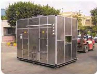
Ammonia Deep Bed Chemical Scrubber
